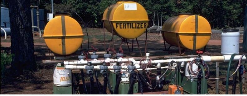
A fertigation unit and valve manifold.
