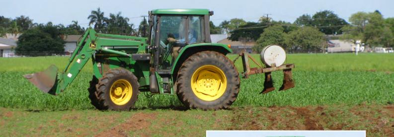
The Wallace Plough is a five typed implement designed to break up hard layers in the soil.
