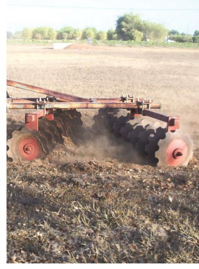
Offset discs can be used to incorporate green manure crops. Keep use to a minimum as they can cause hardpans.
