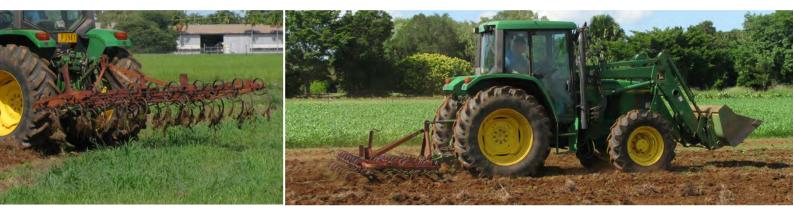
A spring tyned cultivator is used to work up soil with minimal disturbance.
