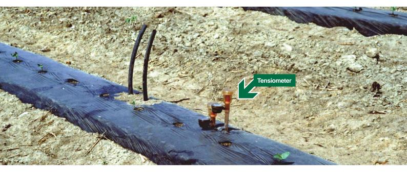
Tensiometers are cost effective and can increase the accuracy of your irrigation management.
