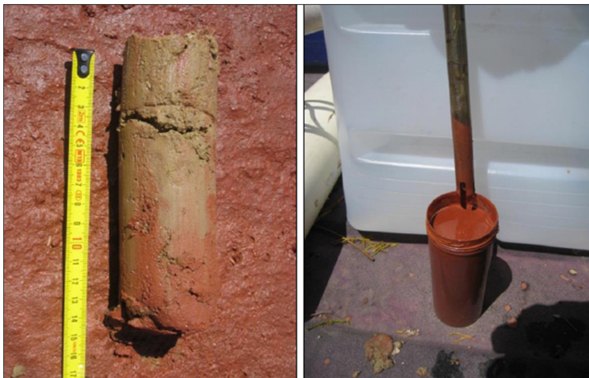
Left: sediment core showing top fraction of iron ore. Right: sediment from Zone 2 in a 1:5 ratio with deionised water. Source: Thorburn, 2015.
