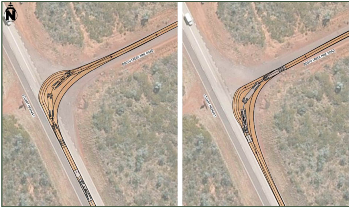
Figure 9 Stuart Hwy/Bootu Creek Mine Rd – Triple Road Train Swept Paths
