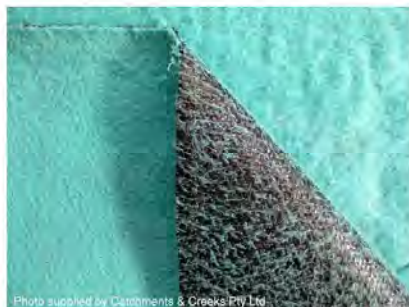
Photo 5 – Composite fabric with the woven (black) backing being the down-slope face of the sediment fence
