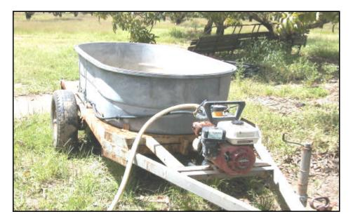
**Figure 7.** A simple fertigation unit comprising a plastic (non-rust) mixing tank coupled to a small injector pump. Trailer mounting allows easy transport to different irrigation blocks.
