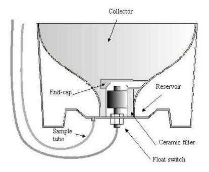
**Figure 11:** The FullStop is a funnel shaped apparatus that is buried in the soil in the rootzone. After irrigation is applied the water percolates through the soil to the funnel that collects the water and closes a float switch that, in turn, provides the signal that irrigation is complete. As the soil begins to dry again, water is drawn out of the funnel which then resets the device for the next irrigation.
