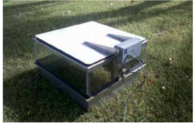
Figure 3. Automated chambers automatically open, close and take samples of gas, which are then analysed on site by electronic sensing devices
