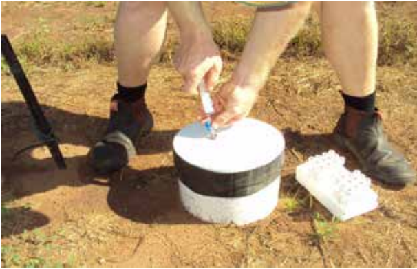
Figure 2. Manual chambers made of PVC are inserted into the soil and are manually closed; during this time gas samples are taken from the chambers and stored in vials for analysis in a laboratory
