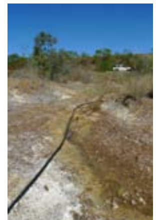
In May 2012, the seepage from the TSF Cell 1 appeared to be fresher than in previous years, as evidenced through the presence of algae and grasses along the drainage line.
