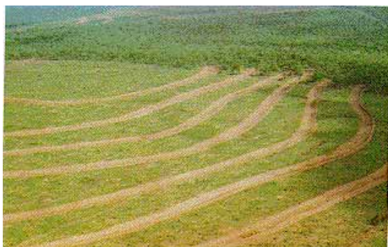
Figure 1. Aerial view of contour banks on land with slopes more than 2%. The closer the banks, the more difficult are tillage operations.
