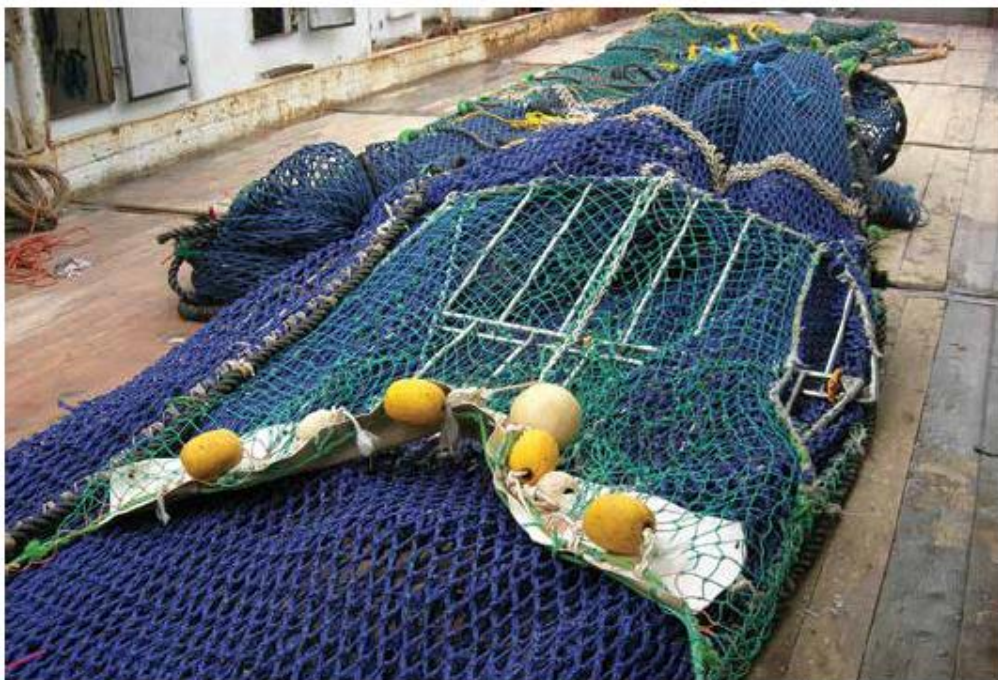
Figure 12. A turtle excluder device on a trawl net used in the Demersal Fishery
