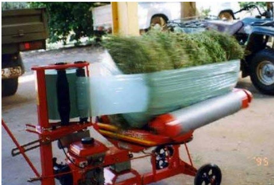
**Figure 3.** A small bale wrapper in operation
