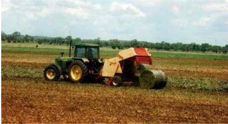
**Figure 1(a).** Cavalcade being baled using a variable chamber baler
