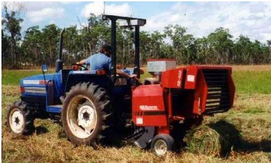
**Figure 1(b).** A variable chamber baler forming small round bales
