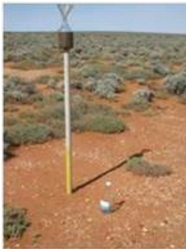
Figure C. Typical deposition dust bottle, field setup on stand, and sample bottle replacement.
