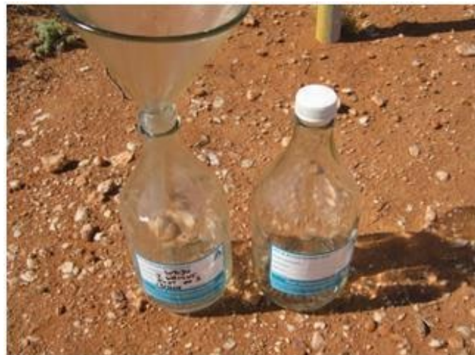
Figure C. Typical deposition dust bottle, field setup on stand, and sample bottle replacement.
