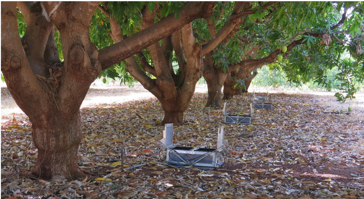
Figure 11. Testing nitrogen efficiency in mango trees with automated greenhouse gas chambers
