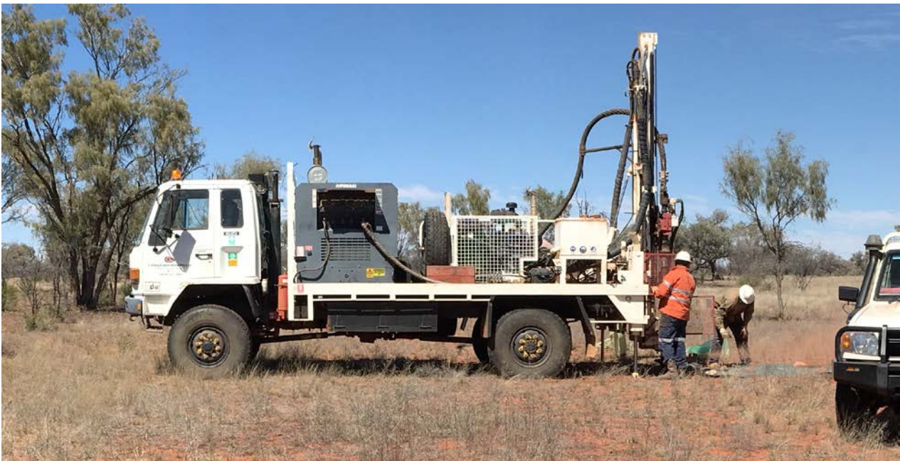
Plate 1: Light weight drill rig from 2016 bedrock geochemistry program
