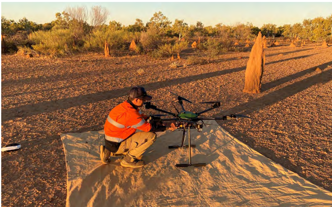
Drone magnetic geophysical survey by Emmerson Resources near Tennant Creek, co-funded through the Resourcing the Territory initiative
