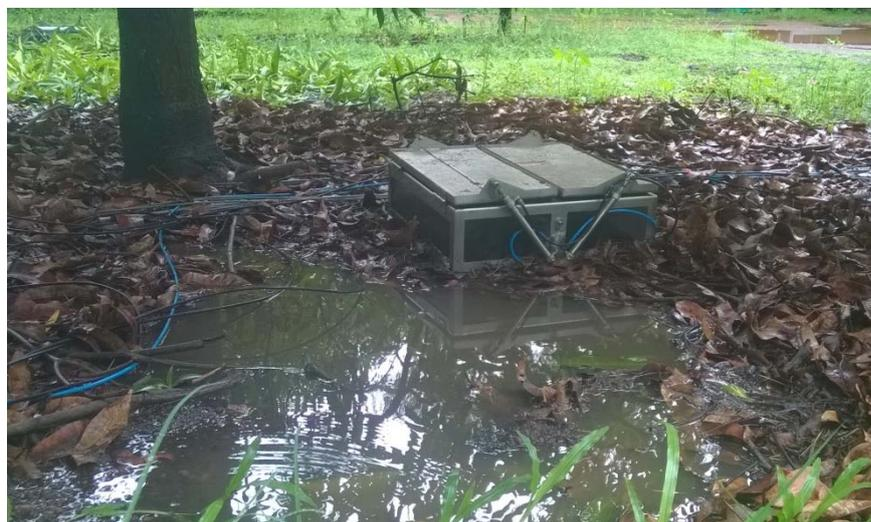
*A fully automated soil gas sampling chamber in a mango orchard after heavy rain. Darwin weather conditions can make gas sampling a challenge!*
