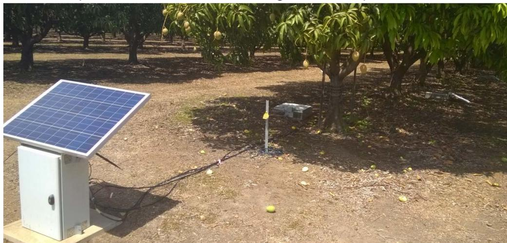
*A semi-automatic soil gas sampling system set up at a Darwin mango orchard. The solar panel and sampler unit are in the foreground, and the sampling chambers are under the mango trees*
