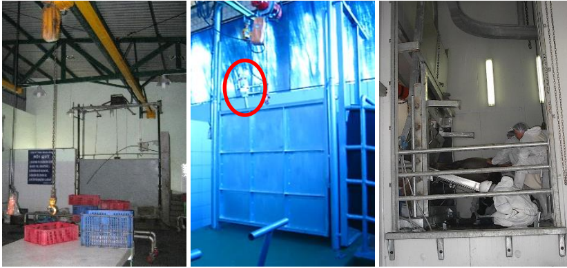
Figure 3.100: (Left to right) Winch-able side panels of knocking boxes (Vietnam, and Indonesia). Note: Stunner hanging above (O); hydraulic side panel with concussed buffalo (Sabah).
