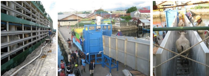
Figure 4.2: (Left to right) cattle boat docked; ramp and transfer box (blue) in place; cattle unloading into truck (Indonesia).
