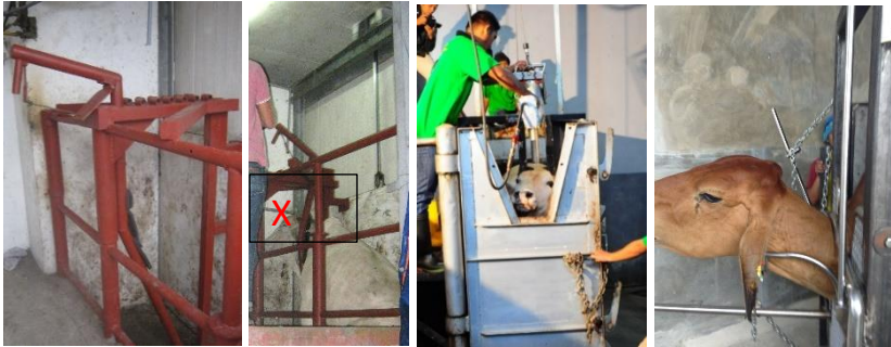
Figure 3.101: (Left to right) Head clamp open; head of electrically stunned animal being released from clamp. Note: Stuning wand (X) Vietnam); hydraulically clamped animal about to be stunned; restraint with chin-lift extension for throat cutting.
