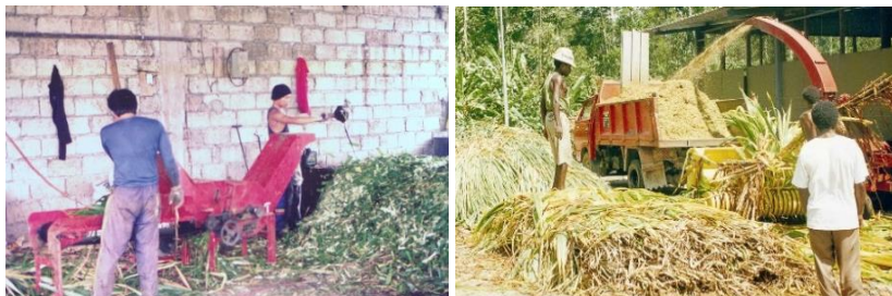
Figure 3.10: Manually operated forage chopper and tractor-operated harvester/chopper.
