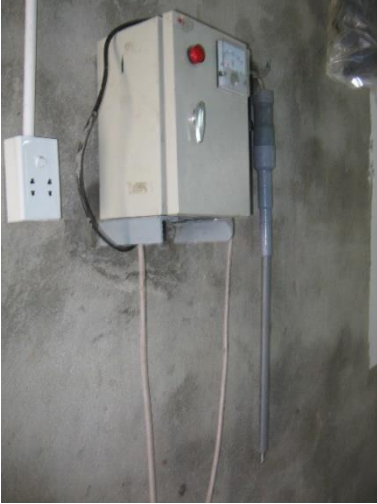
Figure 3.96: Electric stunning power box and wand (Vietnam).
