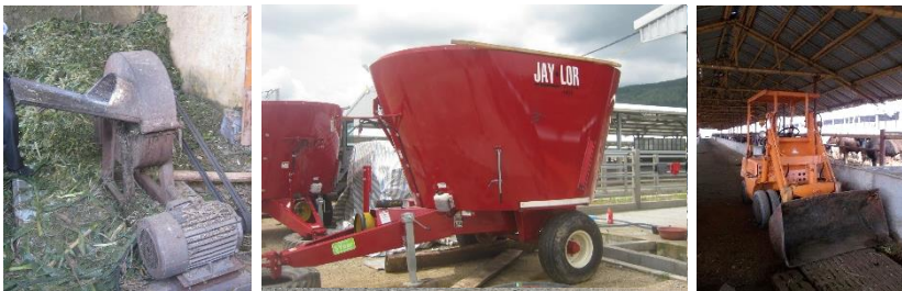
Figure 3.36: (Left to right) Manual loading forage chopper; TMR feed wagon, front end loader (FEL) to remove manure, at Vietnamese feedlots.
