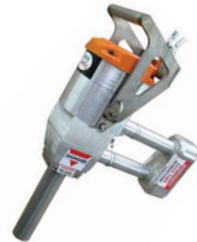
Figure 3.97: Pneumatic stunner (above) and captive bolt stunner (below); both optional as penetrating or non-penetrating.
