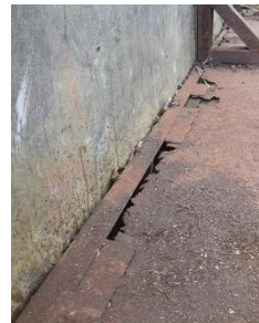
Figure 4.4: Rusty truck floor, unsafe for transportation of livestock.
