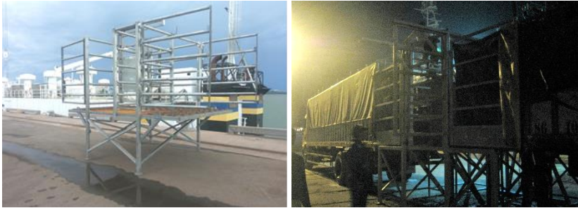
Figure 4.3: (Left to right) SEALS double loading transfer box; loading discharged cattle from ship onto trucks with SEALS transfer box (Vietnam).
